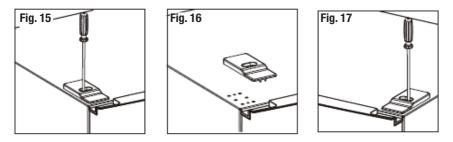
7. Take off the upper door. Remove the screw from the middle hinge using a Phillips head screwdriver. Then take off the lower door. Move the hinge hole covers from the left to the right side.
