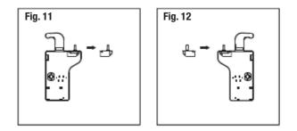
5. Detach the cover of the upper door and move the harness from the right side to the left side, then replace the cover.
