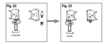
10. Refit the bracket fitting the bottom hinge pin. Replace both adjustable feet.
