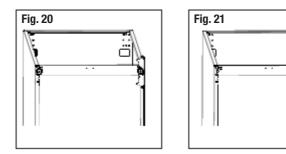
9. Unscrew and remove the bottom hinge pin, turn the bracket over and replace it.
