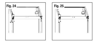
11. Remove the aid-closers from the bottom of the upper and lower doors. Then take the new aid-closers from the hardware accessories bag and install them to the left side.
