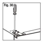
15. Connect the harnesses from the door and cabinet. Then replace the top hinge cover. Before screwing in the cover, connect the terminals of the door switch.
