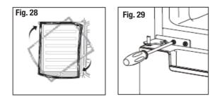
14. When replacing the upper door, make sure to align it with the cabinet to ensure the door gasket seals the cabinet tightly. Then connect the door with the cabinet by tightly fixing the top hinge.
