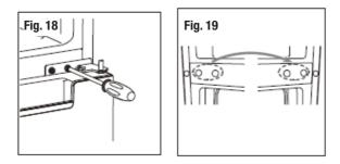
8. Unscrew the bottom hinge. Then remove the adjustable feet from both sides.
