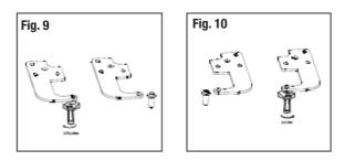
4. Move the door switch from the right hinge cover to the left hinge cover from the hardware accessories bag.
